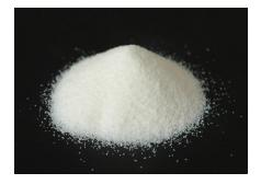
Mr. Genesis is unlike other solidification media, such as sawdust, Portland cement, kitty litter, Dri-Rite or kiln dust, in that it chemically bonds with water. It will hold it under pressure and only add minimal mass.
